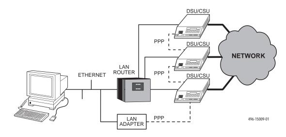
Figure 2-7. LAN Adapter and Daisy Chaining
